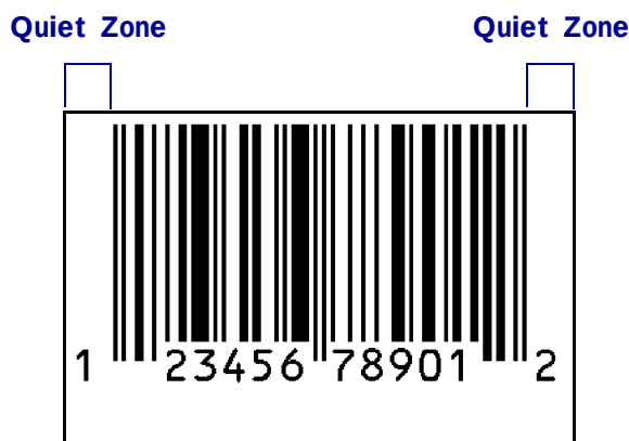
Figure 9 • Quiet Zone in a Bar Code
